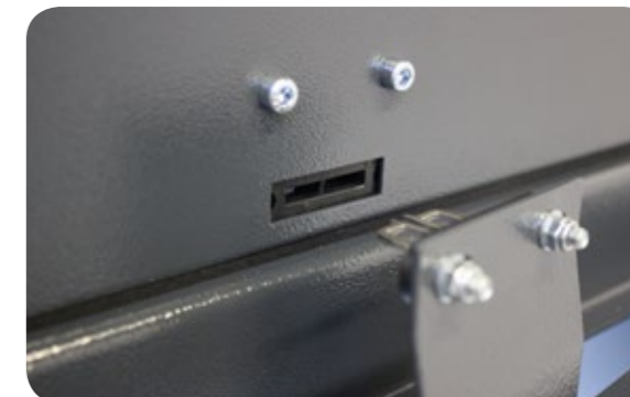
Door safety switches
