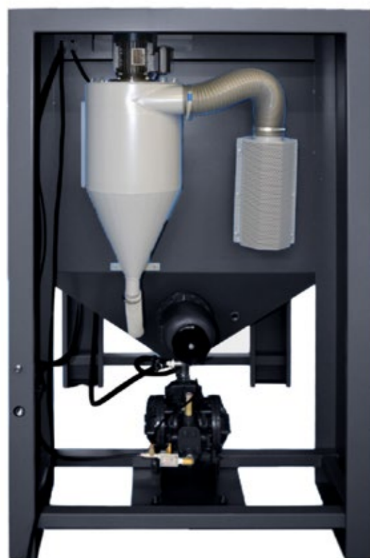
NP12 Wet Blasting Cabinet with cyclone and filter room
