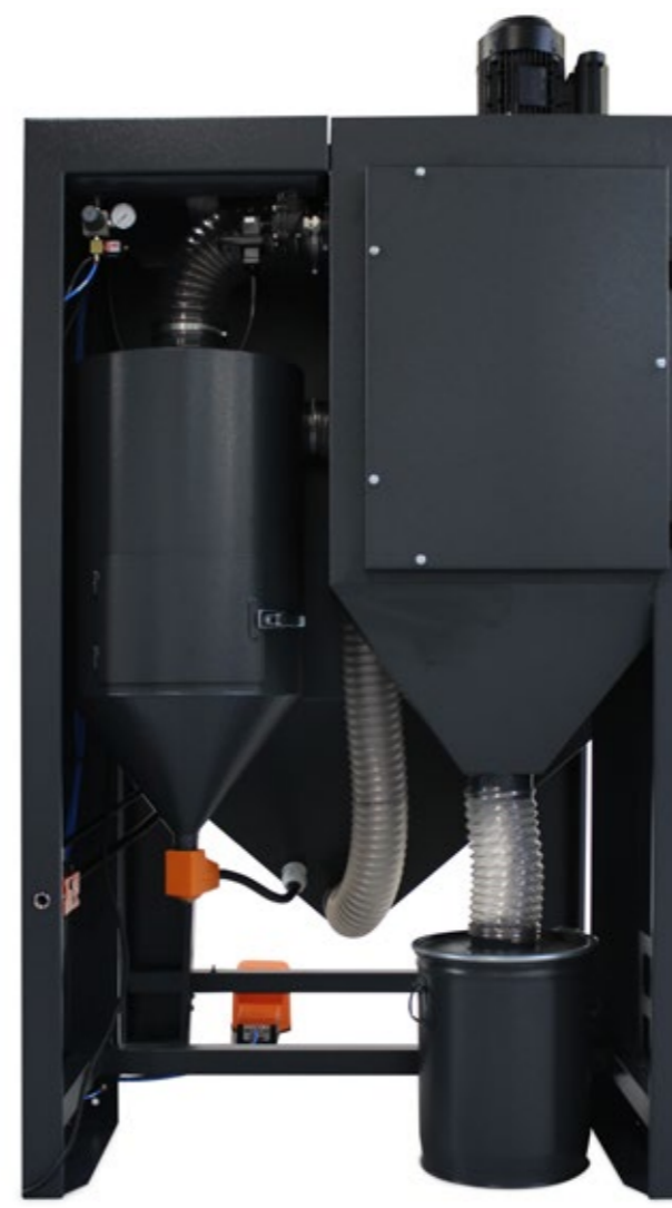
DI12 Suction Blasting Cabinet with cyclone and filter room
