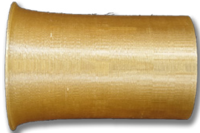
Ra Before: 13.25 \mu\text{m}
